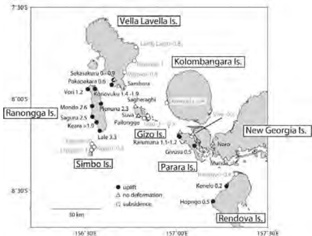
Figure 6-28 Measured ground deformation data around Gizo (from Tomita et al, 2008)
