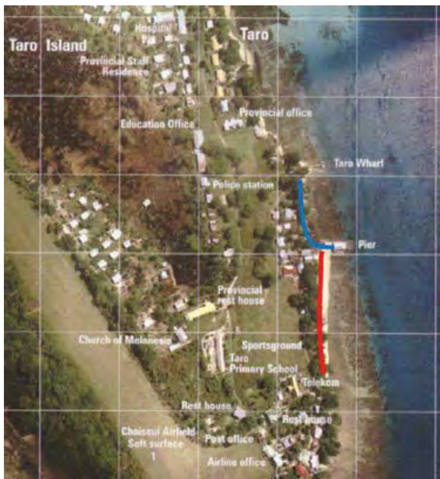
Figure 6-37 Zoomed image of orthophotomap showing evidence of a northward transport and localised erosion as a consequence of pier construction (from 2003 orthophotomap 1-SIOPM-X011)
