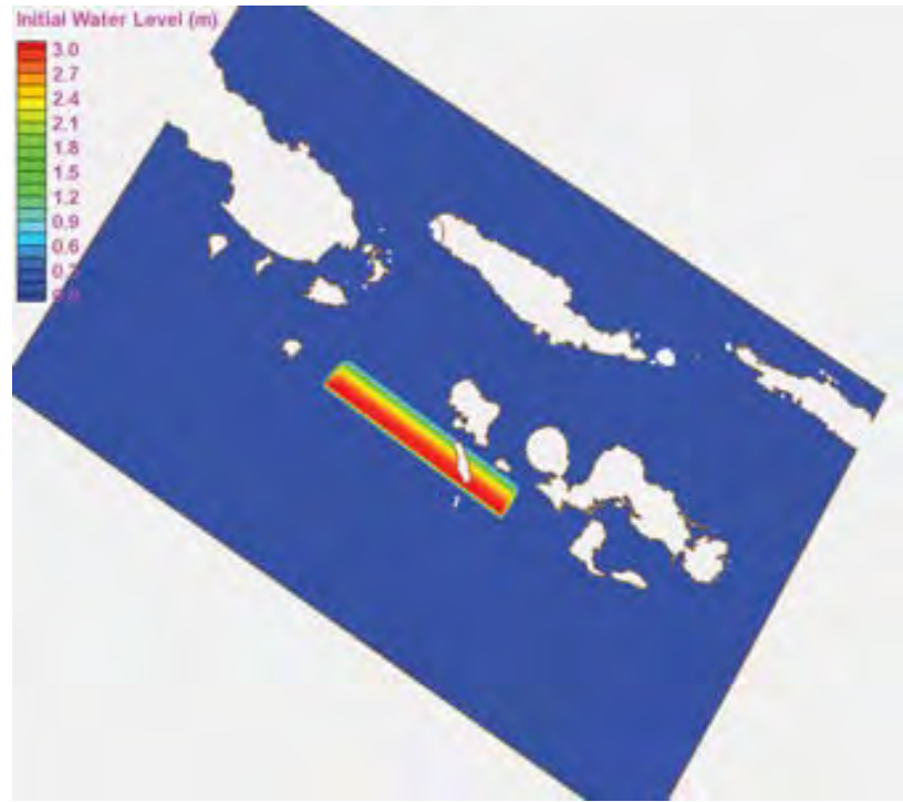
Figure 6-29 Adopted initial water level disturbance - 2007 tsunami event simulation
