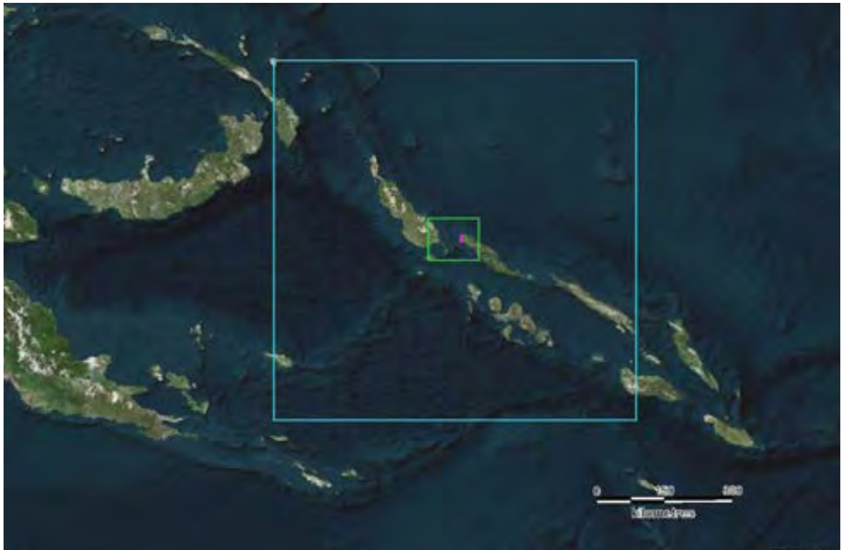
Figure 6-13 SWAN model domains for simulation of cyclone induced wave generation
