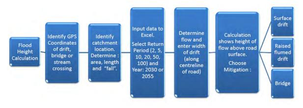
Flow chart for calculating height of flood over drift
