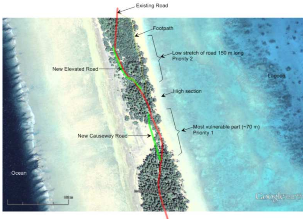
Figure 2.11. The existing road is shown in red – the northern section previously ran along the eastern edge adjacent to the lagoon, where there is now a footpath; it was abandoned due to erosion and over-topping making it impassable during higher tides and large wave events. In the Priority 1 southern areas, the new causeway road will be set some 15-20 to the west of the existing causeway road (shown with the green line) to provide an additional erosion buffer on the eroding eastern side of the causeway. The new elevated road in the northern Priority 2 area will run along its existing route (also shown with a green line).
