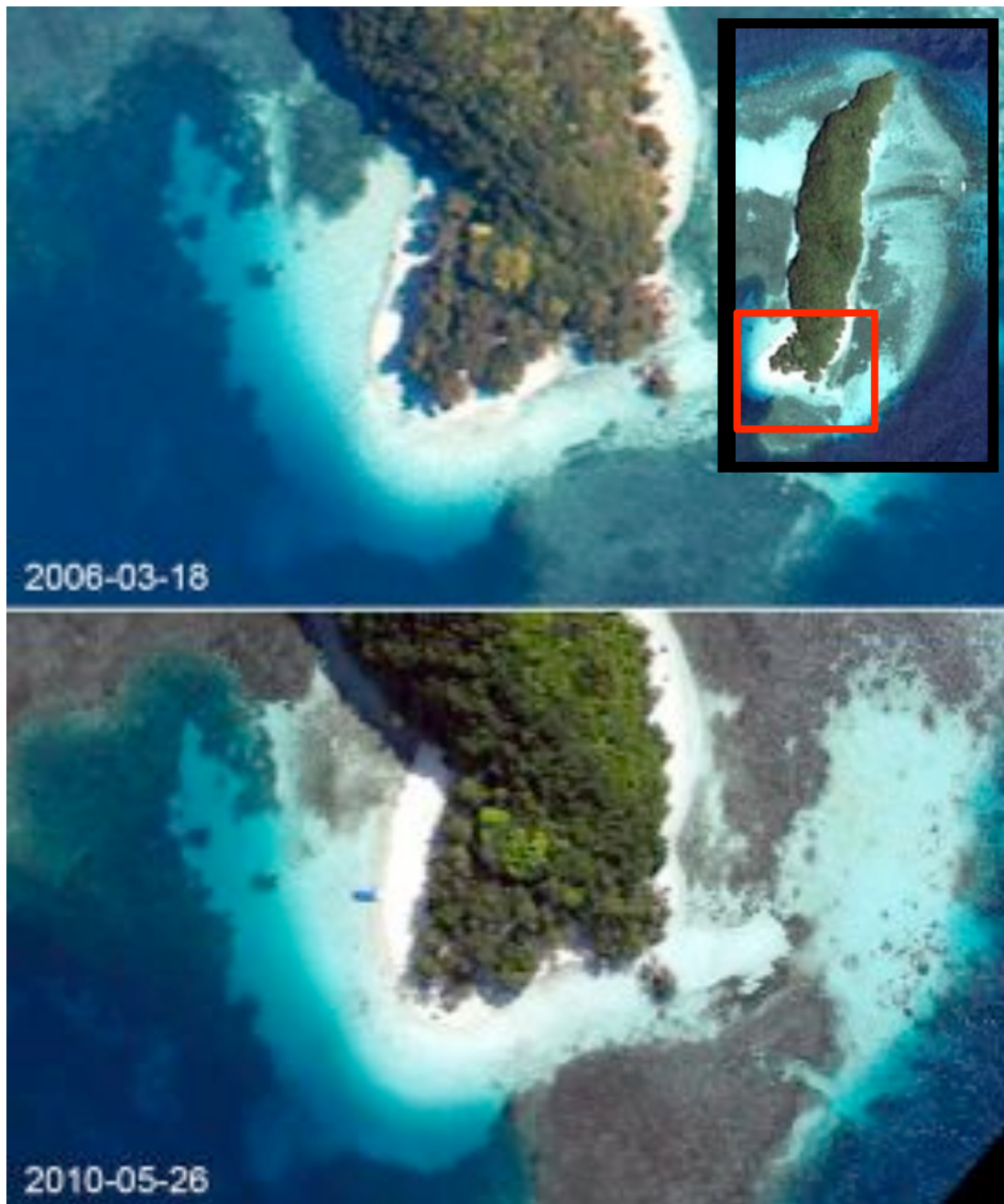
Two images of Ngermeaus Island and tourist beach area in the south. The change in the position of the toe of the beach in the east is easily seen (it's moved landward in 2010) and the western beach (left hand side) has clearly accreted westwards (images sourced from Colin, 2011).
