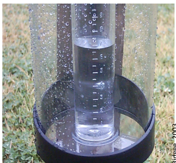
Fig. 4: Rain collected in a rain gauge
