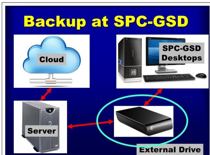
**Figure 02:** Data backup at SPC-GSD. The external hard drives keeping the master copies for the countries. From there servers and cloud backup get synchronised.
