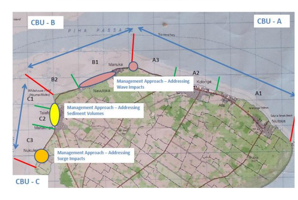
Monitor beach levels and maintain groyne bay volumes to determine amount of littoral drift required for each groyne bay (using beach recycling techniques from Unit C1 or through recharge from offshore sources)
