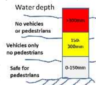
Figure 65 – Warning signage in event of flood
